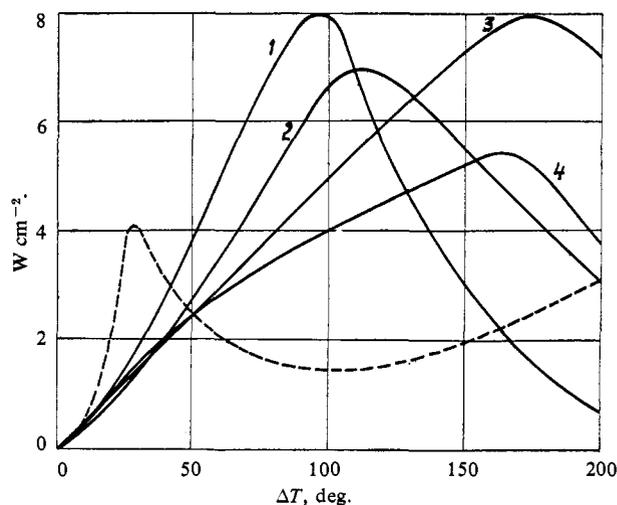
Figure 3. Heat flux density for various thicknesses of varnish layer: (1)  $10 \mu\text{m}$ ; (2)  $20 \mu\text{m}$ ; (3)  $35 \mu\text{m}$ ; (4)  $100 \mu\text{m}$ ; dashed curve, no varnishing.
