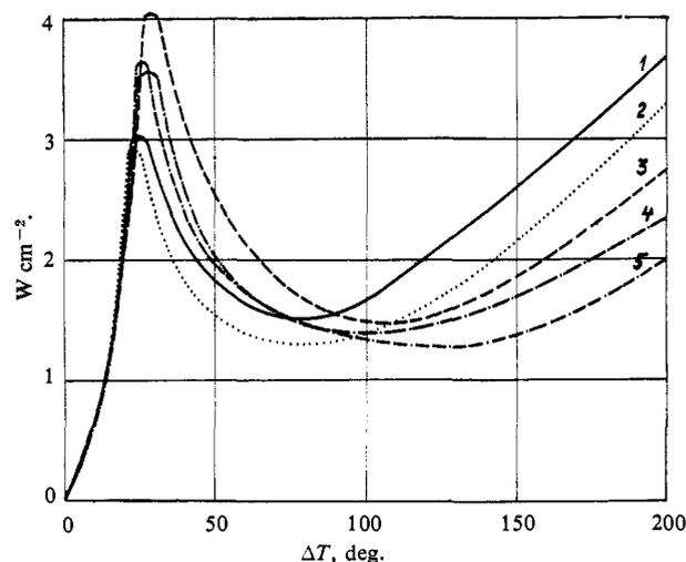
Figure 2. Heat flux density as a function of temperature difference: (1) hydrogen, (2) neon, (3) oxygen, (4) nitrogen, (5) argon.
