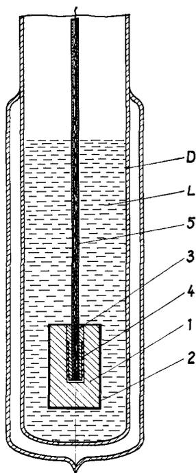
Figure 1. Apparatus: (1) lead block, (2) stainless-steel jacket, (3) inset, (4) resistance thermometer, (5) suspending tube, (D) dewar vessel, (L) liquid.
